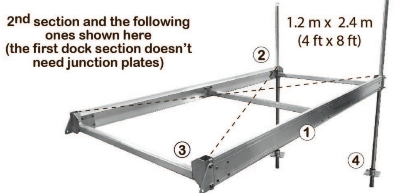
**STEP 2** Insert and bolt in the 2 end pieces with 1/4 in. x 1 1/4 in. bolts by hand (longer part of leg holder on top). You can now tighten all assembly bolts (BEWARE, aluminum is soft – DO NOT over-tighten).
