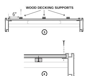
You will assemble the decking panel upside down in order to facilitate your work and you'll flip it back later, so, place decking planks on dock structure "good" side face down, into the dock side support lips, flush on one side, and leave an equal space between each plank (approximately 3/8 in.).
