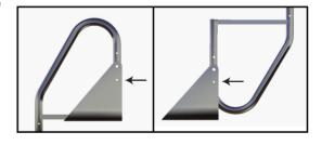
3- Add protection rings and gently tighten the pivot bolts, keeping them loose enough to let the ladder flip.
